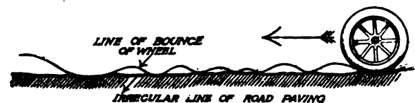
Bouncing action of wheel over rough road.
